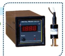
All Pirani Gauges are based on the principle of measurement of thermal conductivity of gases. The Digital Pirani Gauges come with a single gauge head or a dual gauge head enabling the use of one instrument to measure the vacuum of 2 points. The Digital Pirani Gauge is a direct replacement for the conventional Analog Pirani Gagues & is mains operated on Single Phase , 230 V.A.C. supply.
